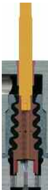
Figure 7. An example of multi-stage, debris-tolerant trim for gas service
