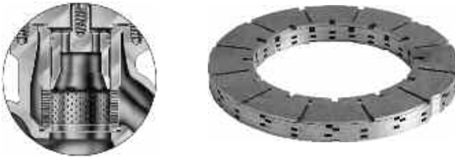
Figure 4. Examples of small passage drilled-hole and tortuous-path control valve trim for liquid service. These would reliably prevent cavitation in clean service applications, but could become clogged if exposed to a flow stream with entrained debris.
