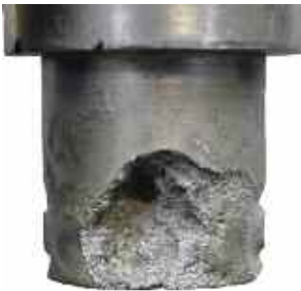
Figure 1. An example of cavitation damage.
