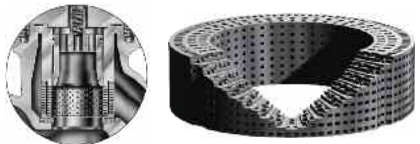
Figure 6. Depicted are small-passage drilled-hole and tortuous-path control valve trim for gas service. These are reliable in clean service applications, but could become clogged if exposed to a flow stream with entrained debris.
